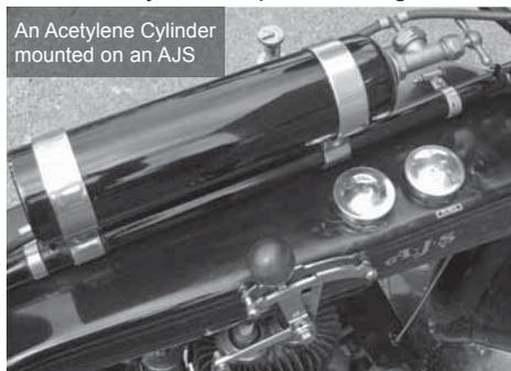
An Acetylene Cylinder mounted on an AJS
