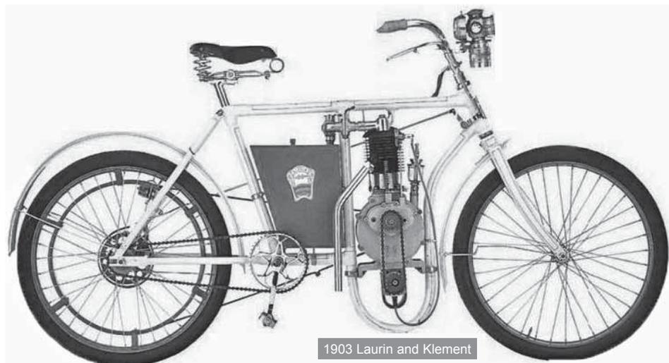
By 1902 Laurin and Klement motor cycles were beginning to attract attention in Britain. Henry Hewetson, a tea trader with interests in Paddock Wood, Kent, imported 150 Laurin and Klement motor cycles which he sold under the Hewetson name. The bikes had a 1¾ hp engine, automatic inlet valve, magneto ignition, surface carburetter, contracting band front brake, optional rear brake and flat or twisted hide drive belt.
